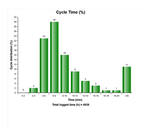
The diagram shows the distribution of the working cycle time. The time between 2 valid cycle registrations is registered. Time starts from lifting the body.
