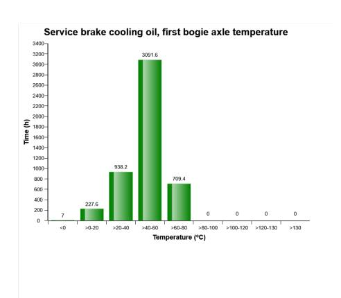
The diagram shows the first bogie axle brake cooling oil temperature. The temperatures are divided into ranges, yellow bar (>120-130 $^{\circ}$ C) and red bar (>130 $^{\circ}$ C) shows abnormal temperatures. The temperature is registered in the line from the first bogie axle to the oil cooler, that is, the warmest oil in the circuit.
