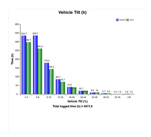
The diagram shows the distribution of the longitudinal tilt in percent (not degrees), the criteria to get registrations is that the vehicle speed exceeds 1 km/h (0,62mph) and that the engine is on.
