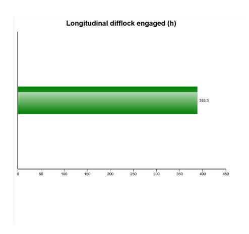
The diagram shows how long time in hours the longitudinal difflock has been engaged. The presentation only shows time when the machine is moving as this is when the wear on the difflock occurs. The difflock should always be disengage when not needed to avoid unnecessary wear.
