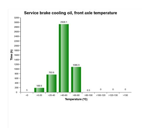
The diagram shows the front axle brake cooling oil temperature. The temperatures are divided into ranges, yellow bar (>120-130 $^{\circ}$ C) and red bar (>130 $^{\circ}$ C) shows abnormal temperatures. The temperature is registered in the line from the front axle to the oil cooler, that is, the warmest oil in the circuit.
