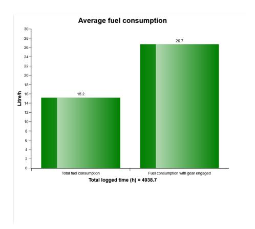
The diagram shows the total average fuel consumption versus average fuel consumption with gear engaged.
