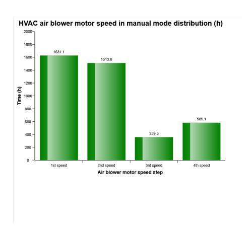
The diagram describes air blower motor speed distribution for HVAC manual control mode established by operator in Cabin.
